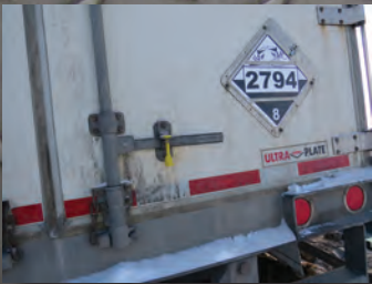
Class 8 Hazard: 50,000 lbs of Batteries
